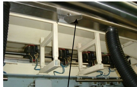
Individual design of the lower manifold considering the movement of the trim box.
